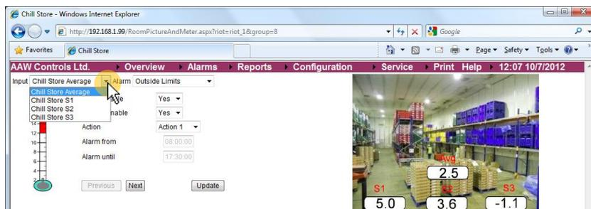
5. The configuration settings for the selected input/alarm are shown.
