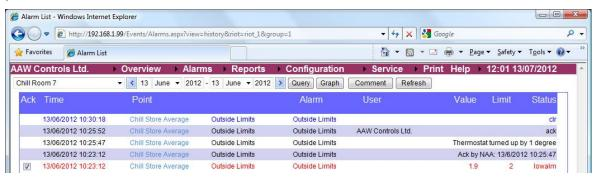
At 10:23:12 on 13/06/2012 the Chill Store was recognised as being below limit for longer than the alarm delay period and an alarm was triggered.
