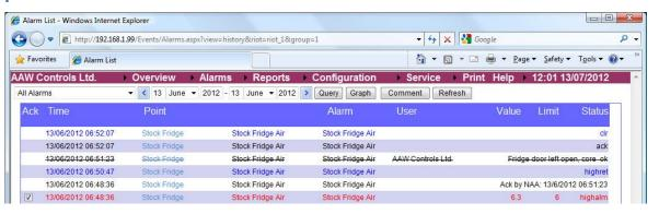
At 06:48:36 on 13/06/2012 the Stock Fridge was recognised as having been above limit for longer than the alarm delay period and an alarm was triggered.
