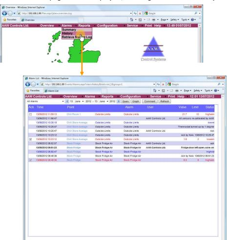
9. To filter the list of alarms/events to a particular room or facility, use the drop down list.
