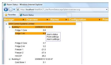
From here the 'Point Settings' (Enabling and disabling points), and 'Alarm Settings' (Adjusting the configuration of an input alarm) can be selected.
