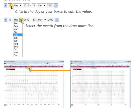
Alternatively, click the left and right arrows on either side of the date range to move the date range forwards/backwards. The sensor graph will be updated automatically i.e. you do not need to click the *Refresh* button.
